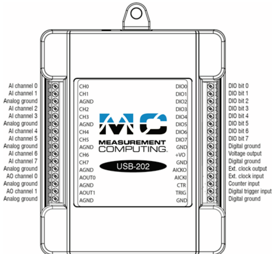
Figure 3. USB-202 pinout
